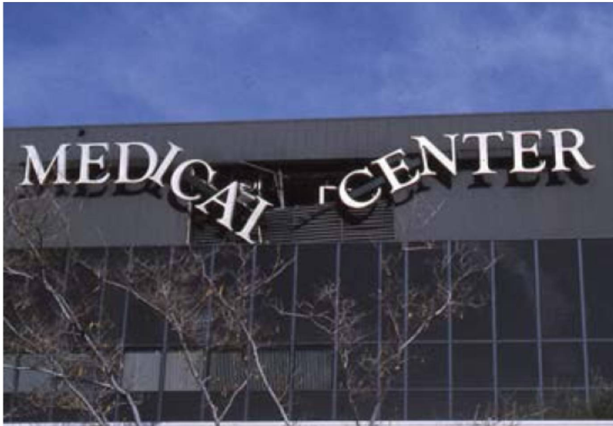
Figure 2. If only the sign on this large hospital had been damaged in the January 17, 1994 M 6.7 Northridge Earthquake, this essential facility could have continued to function. However, the cosmetic damage is an indicator of the fact that mechanical equipment at the top level lurched loose during the earthquake. Without air conditioning, a modern hospital cannot operate, and this one had to close until repairs were made. source: Robert Reitherman (From [14])
